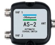
This automatic switch toggles two radios to one antenna. When you key the microphone on one of the radios, it switches the antenna to it automatically. The radio stays locked onto the antenna until the automatic switch detects a transmit from the other radio.
