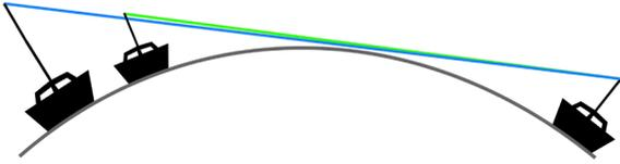
When deciding on an antenna, height is of paramount importance. For clearing low bridges or other obstacles, consider a ratchet-style antenna mount to avoid damaging the antenna..
